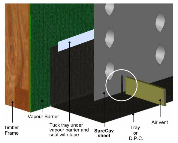
Cut a slot in the SureCav sheet 10mm wide and 65mm high to match the profile of the ventilator (as shown inside the white circle above). If the intended slot does not coincide with the edge of the SureCav sheet then simply drill a 10mm dia. Hole at the top and bottom and cut the material away as shown on the right.
